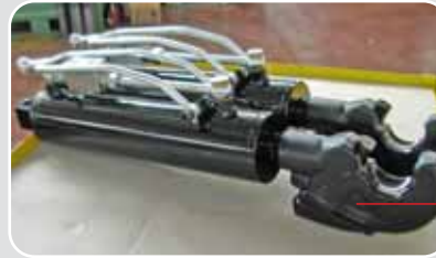
Hydraulic three points linkage with CBM 3 hook NEW HOLLAND
