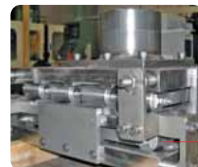
Railway vehicle springs testing equipment
